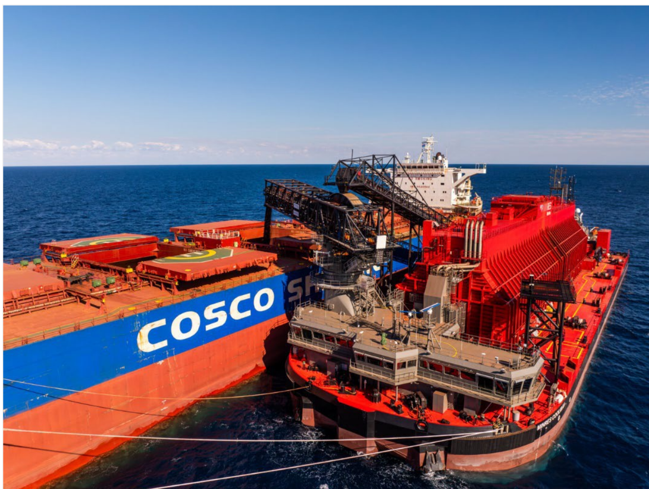
Figure 1: MinRes Transhipper Loading Onslow Iron's First Ore to a COSCO Shipping Bulk Carrier
