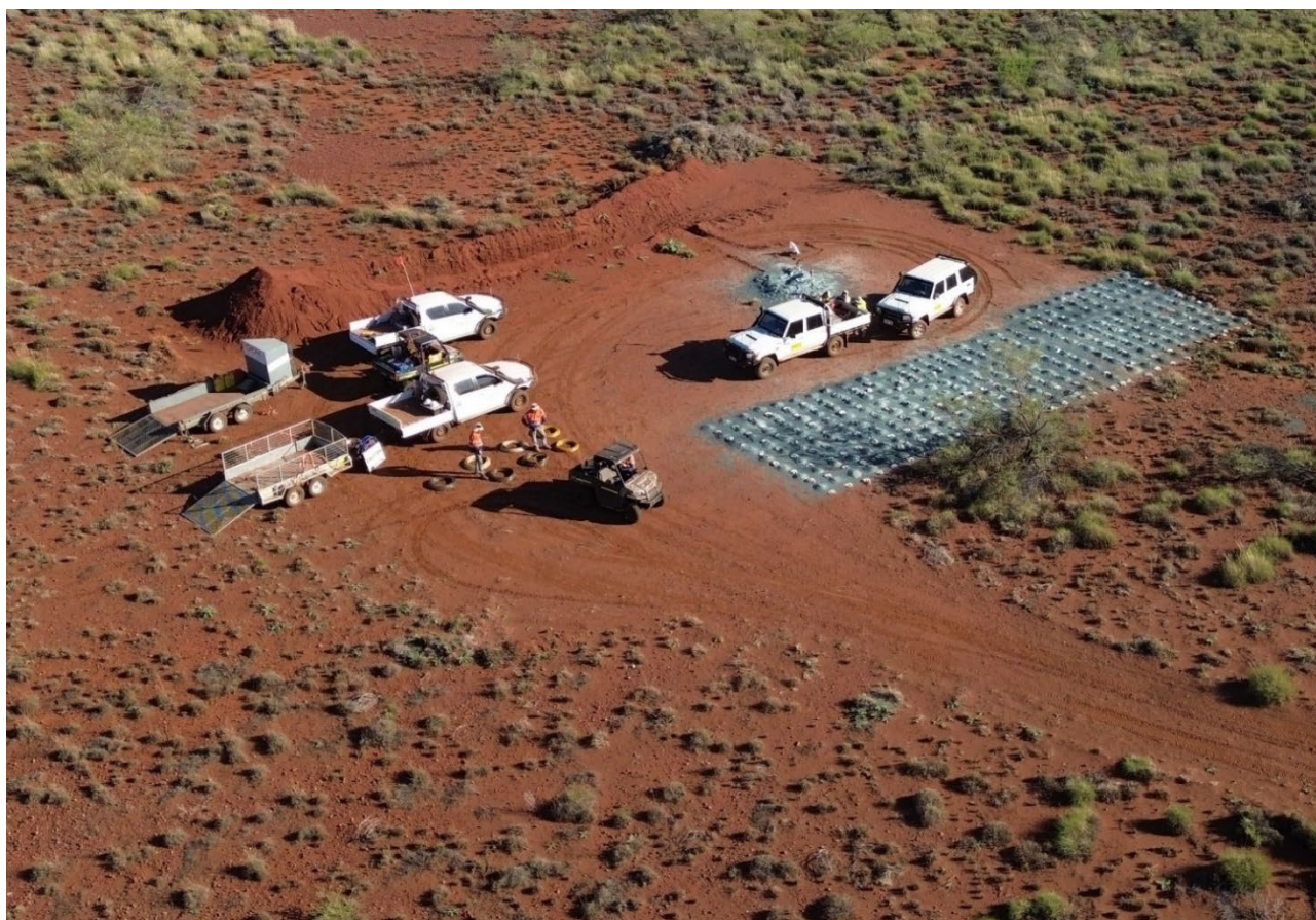
Figure 15: Ground EM survey preparation at Elwood
