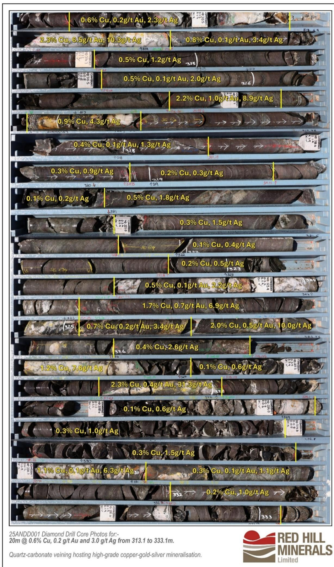
Figure 9: Diamond drill core photos from 313.1 to 333.1 metres in 25ANDD001 that intercepted quartz-carbonate veining hosting high-grade copper – gold - silver mineralisation
