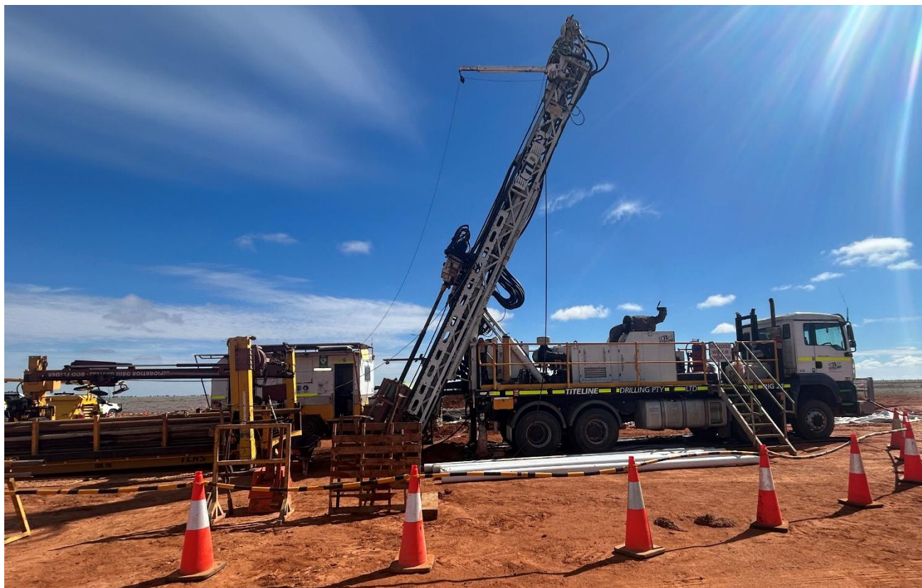
Figure 1: The diamond drill rig setup at the Dementus BHT lead-zinc-silver Target on drillhole 26DMDD001
