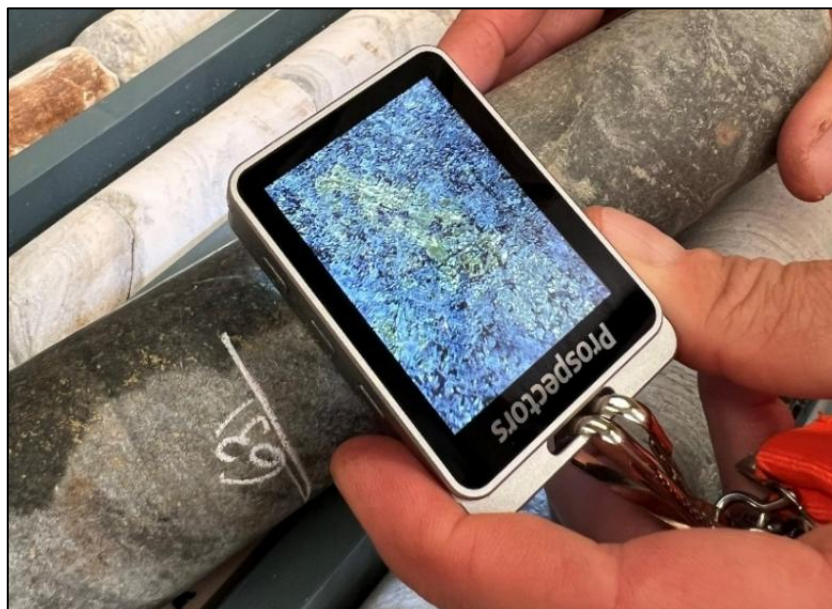
Figure 1: Disseminated sulphide mineralisation in the newly identified dolomitic unit and the underlying Boucaut Volcanics, including chalcopyrite at 631 metres in 26ANDD002 (x10 magnification)
