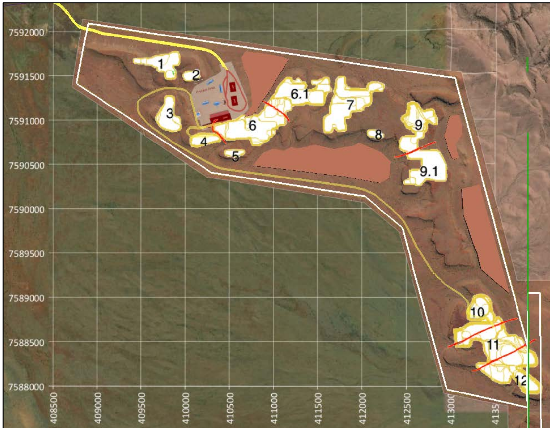
Figure 1 Redgate pits and dumps locations showing sub-pits for scheduling
